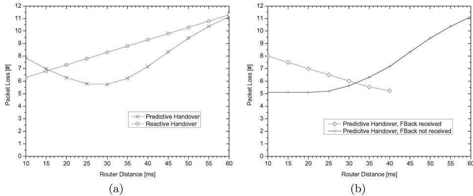
Figure 8. Packet loss during a predictive handover composes from different mechanisms of the scheme: (a) Simulated complete loss for mean anticipation time of 50 ms, (b) contributions from complete and incomplete handover negotiations as functions of access router distance.
