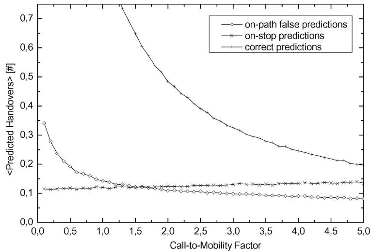
Figure 14. Detailed view on handovers: Correct predictions, failures along the path and on stop.
