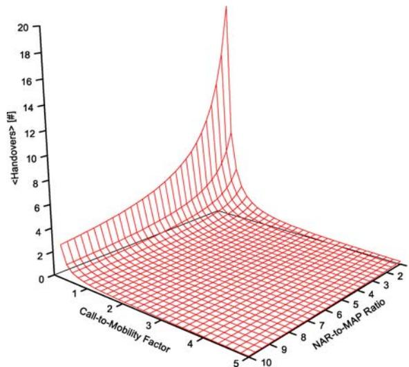
Figure 9. Expected number of handovers as function of the call-to-mobility factor and the ratio of access routers to MAPs.
