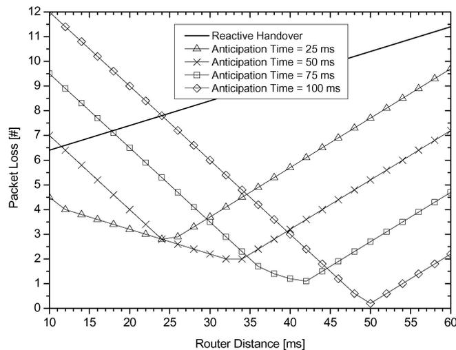
Figure 5. Analytical packet loss in predictive handovers as a function of access router distance.
