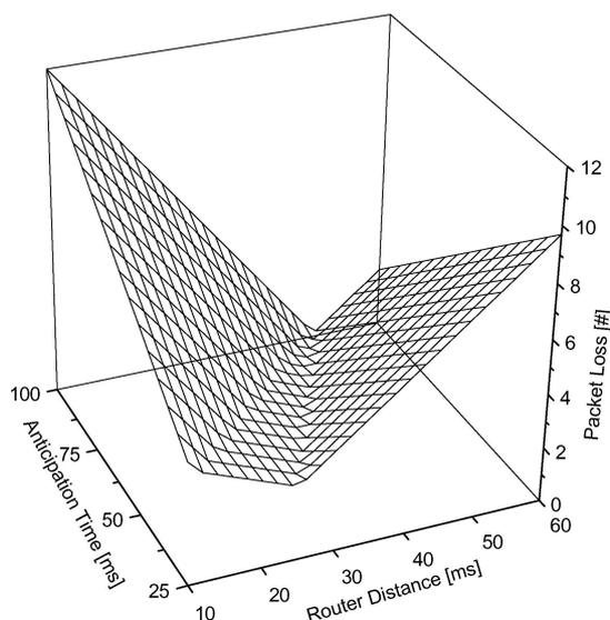
Figure 4. Analytical packet loss in predictive handovers as a function of anticipation time and access router distance.
