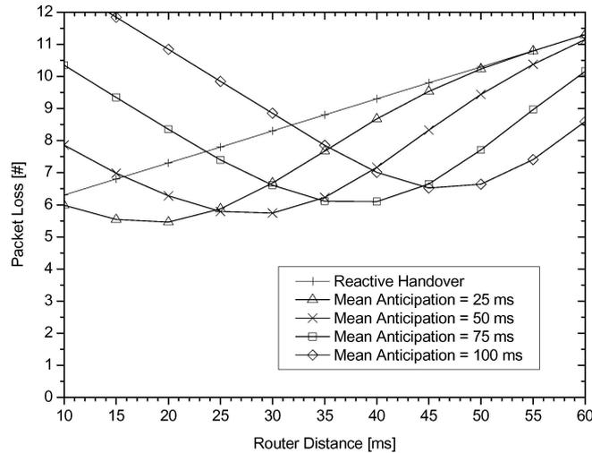
Figure 6. Simulated packet loss in reactive and predictive handovers for various mean anticipation times as a functions of access router distance.
