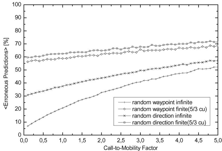
Figure 12. Mean relative yield of erroneous predictions as a function of the call-to-mobility factor for varying transmission ranges.
