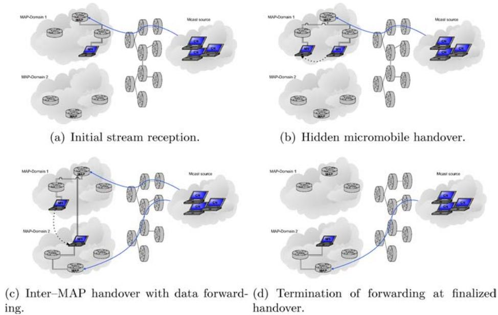
Figure 1. Multicast handover for M-HMIPv6 receivers.
