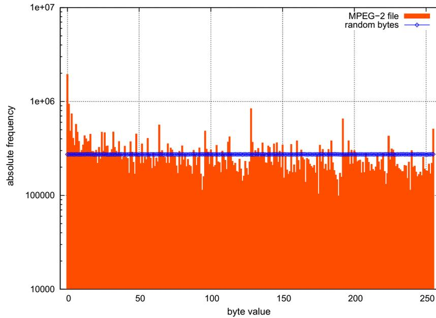
Fig. 6. Comparison of a pseudo-randomly generated file with a not encoded MPEG-2 video stream.
