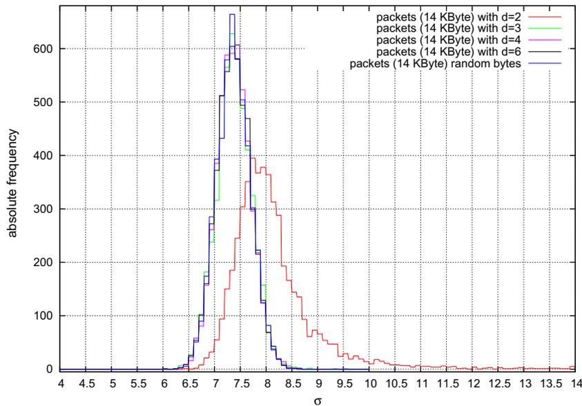
Fig. 4. Comparison of encoded packets with different degrees (no compression).
