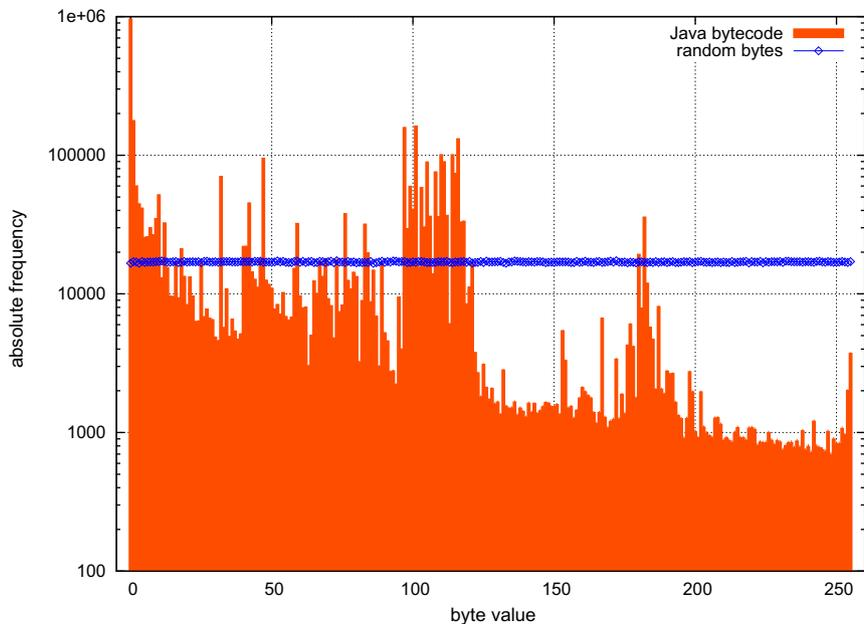
Fig. 9. Comparison of a pseudo-randomly generated file with Java bytecode.
