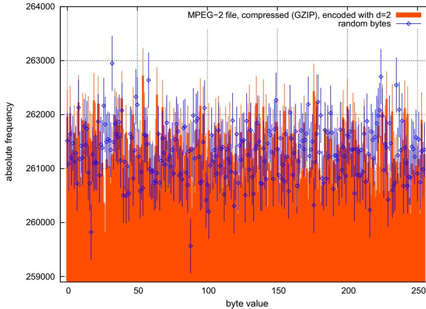
**Fig. 12.** Comparison of a pseudo-randomly generated file with a compressed (GZIP) MPEG-2 video stream purely encoded with  $d = 2$ .
