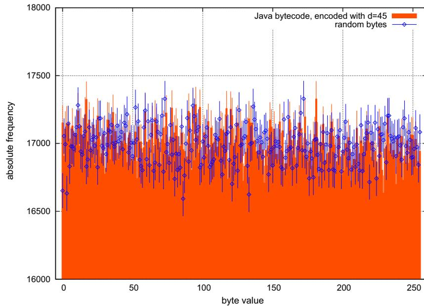
Fig. 11. Comparison of a pseudo-randomly generated file with an encoded Java bytecode ( $d = 45$ ).
