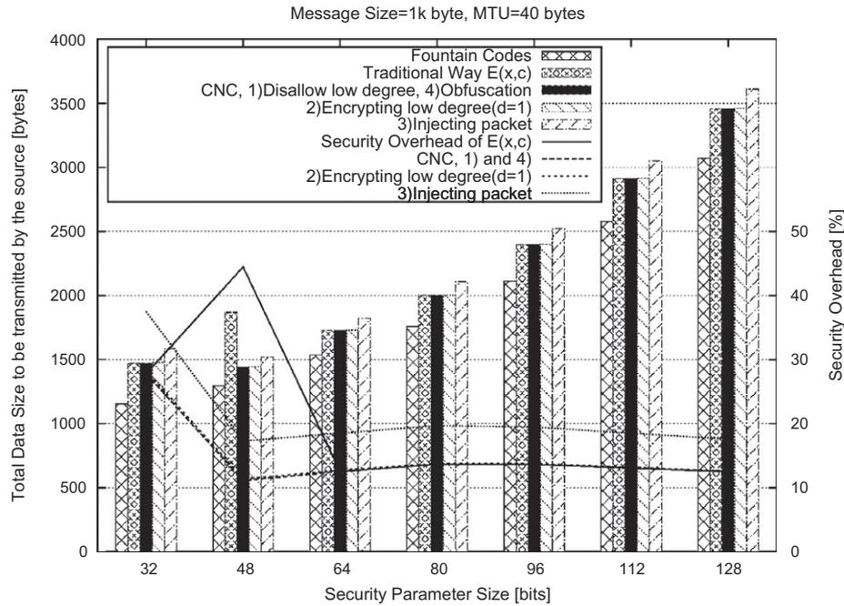
**Fig. 3.** Communication costs (in bytes) and security overhead comparison when 1k byte data is transmitted by the source and MTU on a layer of a communications protocol is 40 bytes.
