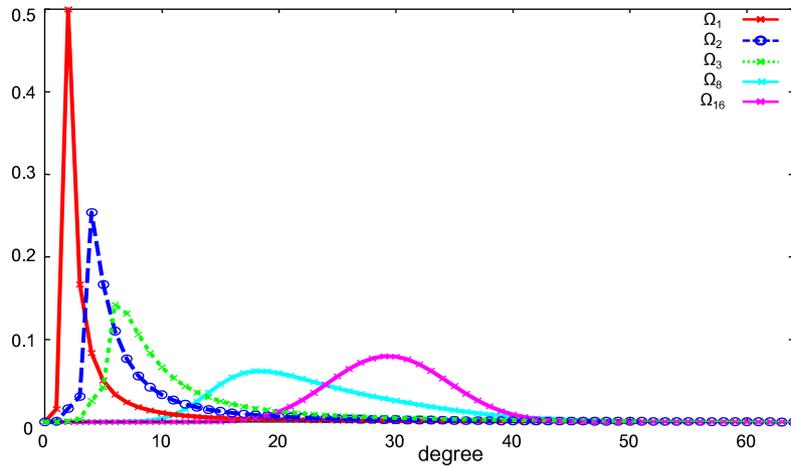
Fig. 1. Degree distribution degeneration of encoded packets due to in-network combination ( $n = 64$ ).
